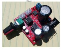
We recommend separate volume controls for this reason. and they should be placed in the signal path before the pre-amps. This is easy if you purchase the volume potentiometers that come pre assembled on a board with two JST connectors. You can of course just buy the potentiometers and either place them on a small piece of PCB with JST connectors or alternatively cut a JST cable in half and soldering them direct to the pot.
